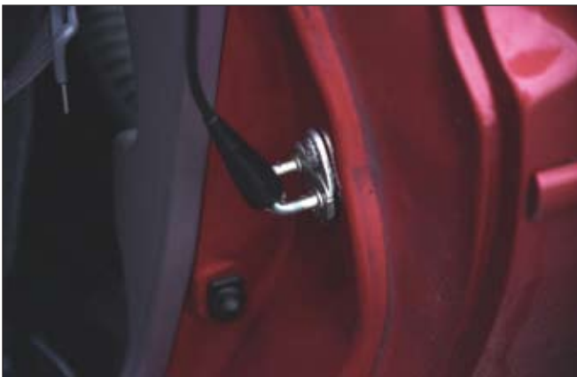
Figure 6: Example of Proper Vehicle Grounding
